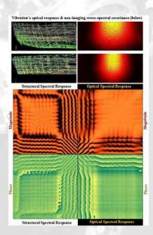
Tank armor nonlinear clattering sensed by laser imaging. Time evolution of modes analyzed for covariance of the spectra – structural (left) vs. optical (right) for magnitude (copper) vs. phase (green). "Laser Covariance Vibrometry ..." thesis.
